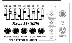
Set the FIELD EFFECT CHANNEL rotary controls and the 9 Band Graphic E.Q.
